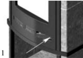
1. Remove excess (not all) ashes. NB, there can still be glowing embers after more than 24 hour after initial lighting. Always empty ash remains into a fireproof container.
