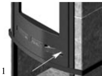
1. Insure maximum airflow by opening the air valve.
