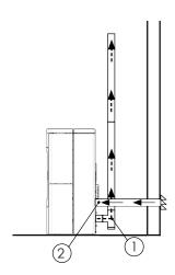
smoke discharge (1) and oxidising air channelling
