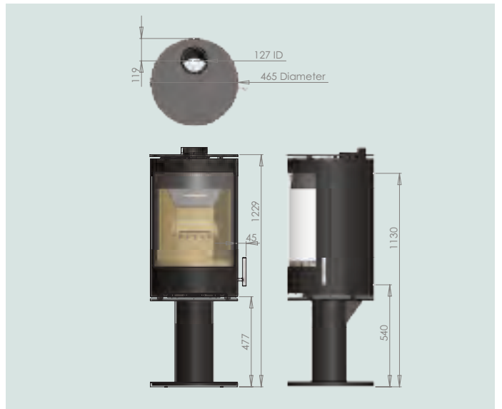
PVR cylinder assembly with high pedestal stand
