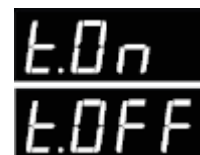
Display of the room temperature thermostat state
