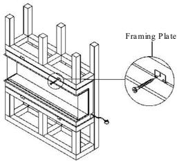
Cladding the framework note: hard surfaces can amplify sound consider adding some underlay or similar to the inside surface of the cladding
