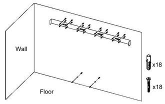
Mount the appliance carefully on the hooks of the wall bracket, secure the appliance To the wall bracket with the screws provided, one into each end
