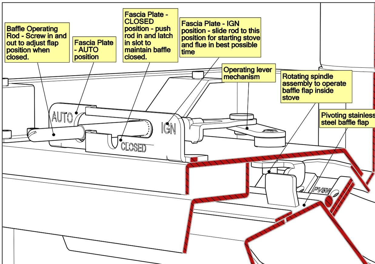
**8.1 Description:** The Purevision range, including the Classic versions may be fitted with an internal stainless steel active baffle assembly which fulfils a number of functions:
