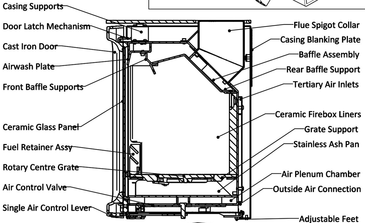
**Fig 2 – Purevision Stove Assembly and controls. 5kW model shown.**
