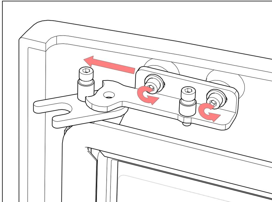
**9.12 Adjusting Latch Pins (mounting on stove body).** The latch pin can be adjusted to enable the latch assembly on the door to catch fully. Firstly slacken the mounting
