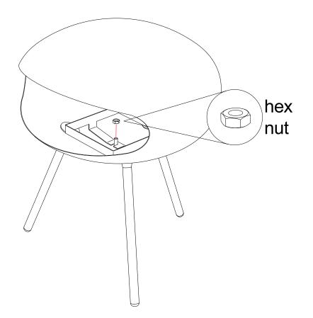
With the Legs securely attached to the Main Body, place the Removable Tray Bracket over the threaded stud at the base of the Main Body, and then tighten in place with the hex nut supplied to be "finger tight". Now follow the adjustment procedures on the following pages before securing with an appropriate tool.
