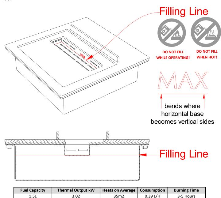
To fill the Combustion Chamber, remove it from the Main Body using the Lifting Handles and pour fuel inside the Vent Opening being careful not to spill. Fill up to the fill line as indicated in red with no more than 1.5L of fuel (3-5 hrs burning time). After filling is done, wipe away any spilled or excess fuel before returning the Combustion Chamber to the Mount Plate opening.
