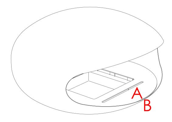
By finely adjusting the *Removable Tray Bracket* backward and forward (1) allows for the necessary adjustment in height (2) of the *Mount Plate*.
