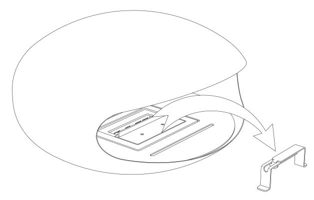
Your Cocoon Burner is now ready to use, follow the steps on the following pages to correctly and safely fill, ignite, adjust, shut off and refill the Combustion Chamber. Always make sure the Lifting Handles are removed from the Combustion Chamber as shown above when it is not in use otherwise these parts will become too hot to touch and may cause injury.
