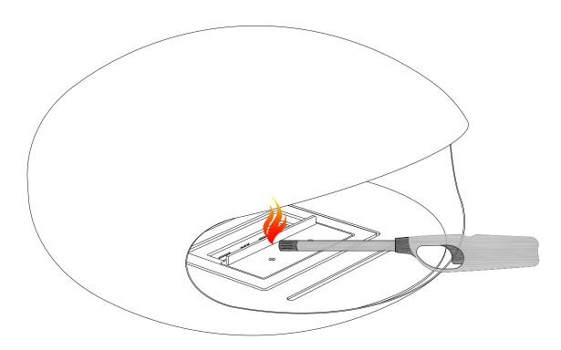
Using a long arm fire lighter and standing at a safe distance from the Combustion Chamber carefully introduce a flame as indicated above to ignite the Combustion Chamber. Always make sure there is a Class ABE fire extinguisher close at hand when igniting the Combustion Chamber.
