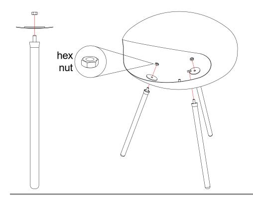
Screw the three Legs from the bottom of the Main Body and secure Legs from the inside of the Main Body with the three hex nuts.
