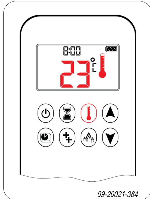
**ON:** Press the [**Thermostat**] button. The symbol is displayed, the pre-set temperature is briefly displayed, and then the room temperature
