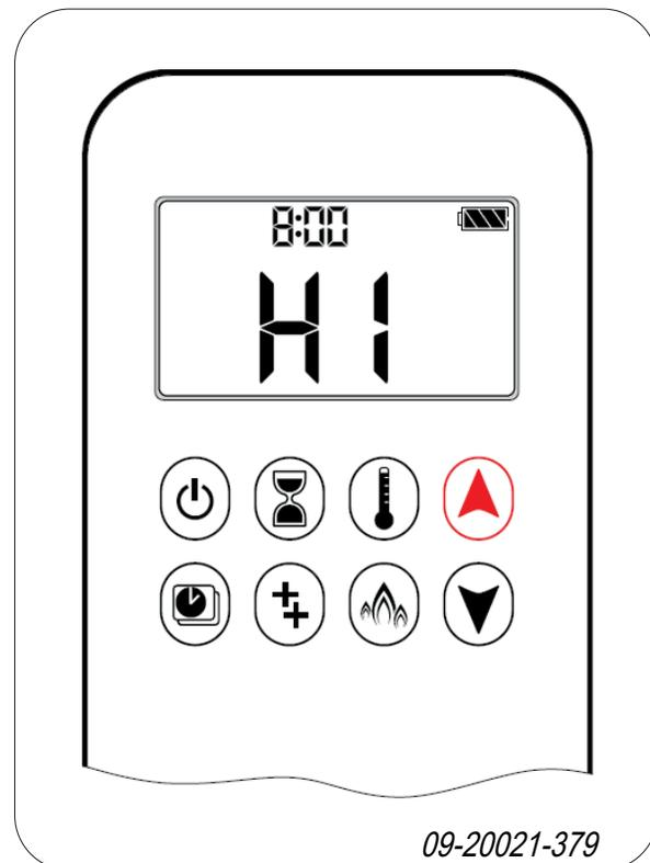
Double-click the ▲ button to switch to high flame. HI appears on the display
