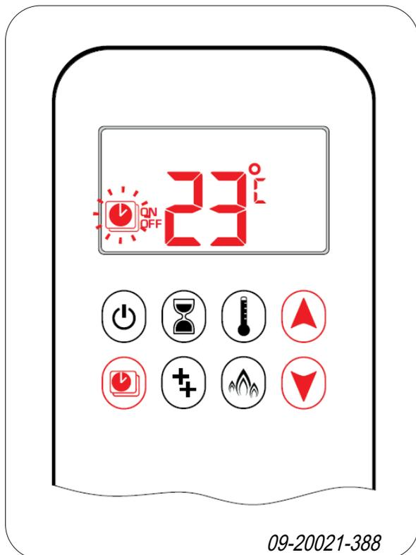
1. Hold down the [**Programme**] key until the symbol starts blinking. ON and the ON temperature appears.
