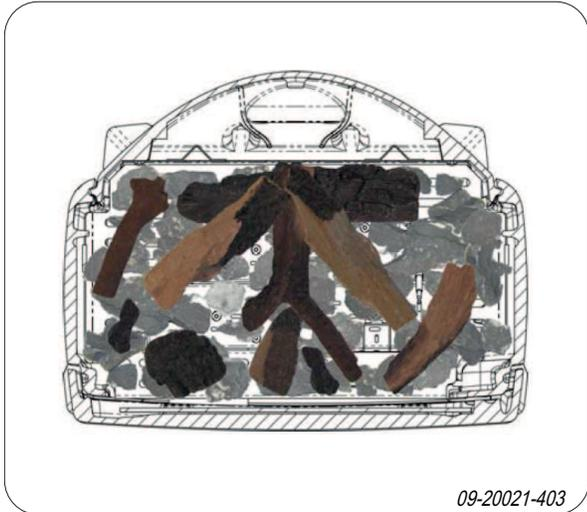
**i** The way the ash granules are spread over the burning surface partly determines the flame effect. In certain cases it may be necessary to change the distribution of the ash granules by partially freeing up several burner openings, for example, in order to improve the flame effect.
