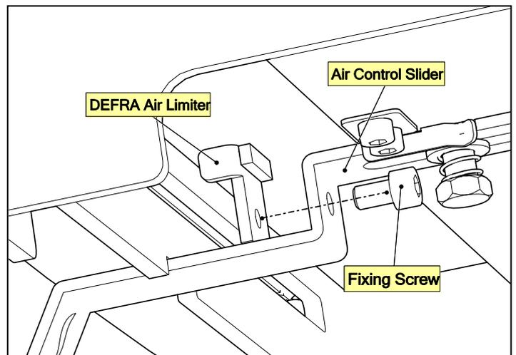
**8.8 Maintenance of air control valve.** The main air control valve is mounted underneath the air plenum chamber which is immediately beneath the firebox base. To access this for thorough cleaning firstly remove the base outside air box. Invert the firebox for access. To remove the outside air box remove 4 x fixing screws from the bottom of the firebox. Now remove locking nuts and springs from the control lever and lift the slider off. Replacement is the reverse of disassembly.
